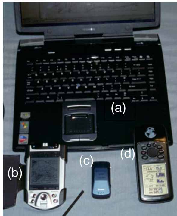
Figure 2. Equipment used for mobile mapping. (a) notebook computer running ArcGIS (version 9); (b) iPAQ handheld computer (5400 or 2700 series) running ArcPad (version 6.0.2); (c) Fortuna “Clip-on” Bluetooth GPS; (d) Garmin GPS 72 Receiver
