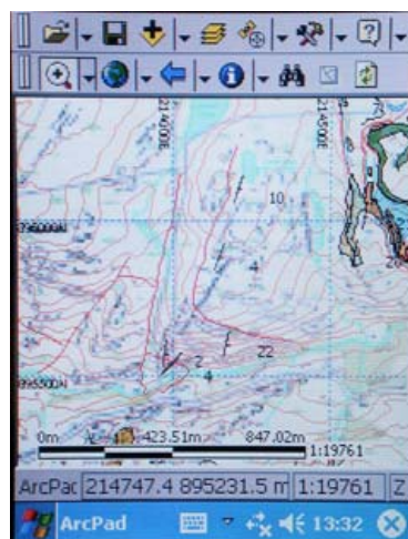
Figure 14. Emulation of exposure mapping using ArcPad. Captured screen image showing “green-lining” of exposed rock and proper representation of geological symbols in the field as measured in the field – an essential part of the geological mapping technique that must be emulated by the digital approach
