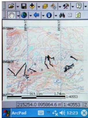
Figure 8. Screen image captured from Arc Pad showing a simple line representing a geological boundary. The grey dots are locations where data (lithology, dip and strike) are stored as shapefiles.
