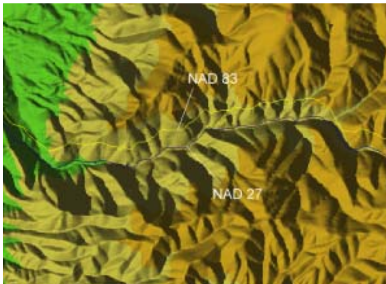
Figure 6:GPS also allows opportunities for calibrating Datums to the UTM DEMs. NAD 27 seems to fit better, by about 100m, than NAD 83.
