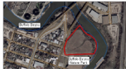
Figure 6. The site has been built up from its original surface configuration by the deposition of construction debris and excavated clay from the burying of pipes under the streets.
