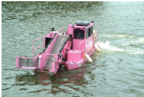
Figure 3. The Mighty Tidy is a skimmer boat purchased to help clean the floatable debris from the waters of the Bayou.
