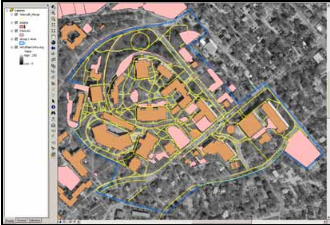
Figure 6 An example of a group's area with their group's boundary (blue), building footprints (light red), parking lots (dark orange), and digitized sidewalks & pathways (yellow),
