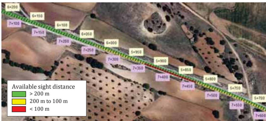
Figure 6. Thematic map representing available sight distance along a short section of a rural road.
