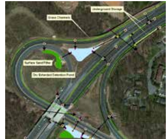
Linked stormwater features
