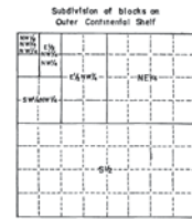
Typical method of subdivision of the blocks, each subdivision being an aliquot part of the total, based on mid-point subdivision throughout
