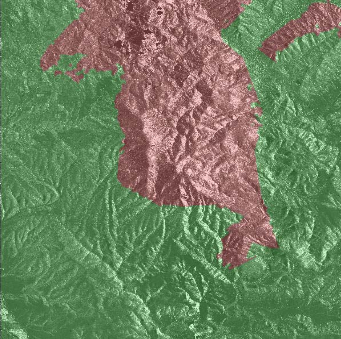
Figure 7. Specific editing guidelines exist for data in targeted versus non-targeted areas. These guidelines are in place so that a more extensive edit is completed in targeted areas. In this example, approximately 2/3 of the mapsheet designated targeted. IV&V uses ArcGIS to examine whether or not editors are editing appropriately throughout the mapsheet with regard to the Target-Editing mask. The first step involves locating where editors have actually modified the data. Subtracting the input or unedited DSM by the edited DSM and then querying all values not equal to 0 accomplishes this
