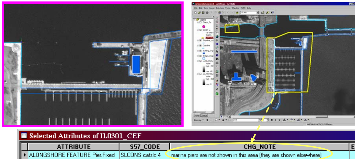
Figure 3 - Imagery is georeferenced to line up with the ENC, and discrepancies are logged in the Chart Evaluation File.
