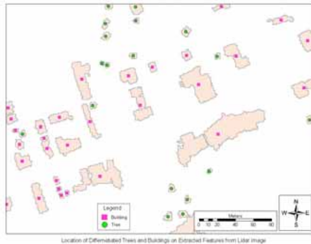
Figure 7. Feature centroids matched to extracted feature footprints.
