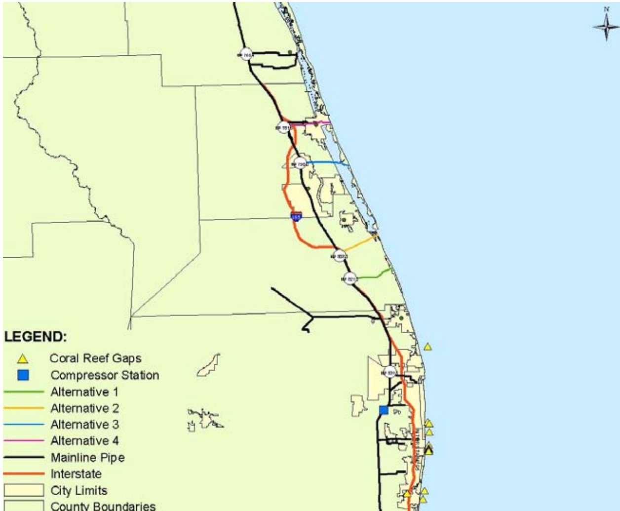
Figure 2. Potential on-shore alternative pipeline routes for a proposed off-shore pipeline.
