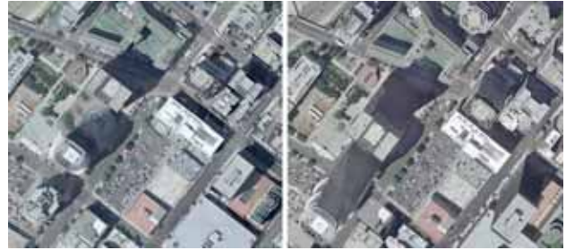
Figure 9. Los Angeles True-Orthophoto (left) compared with Orthophoto (right). True-Orthophoto generation by CyberCity AG. Aerial images by Sanborn Inc.
