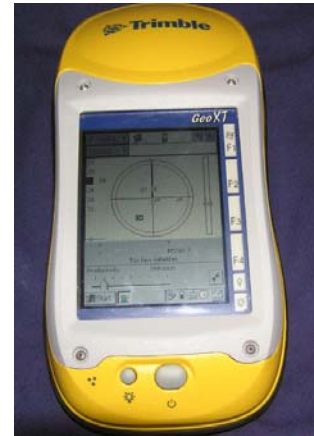
Figure 11. Trimble GeoXT GPS receiver used for data collection during the field test
