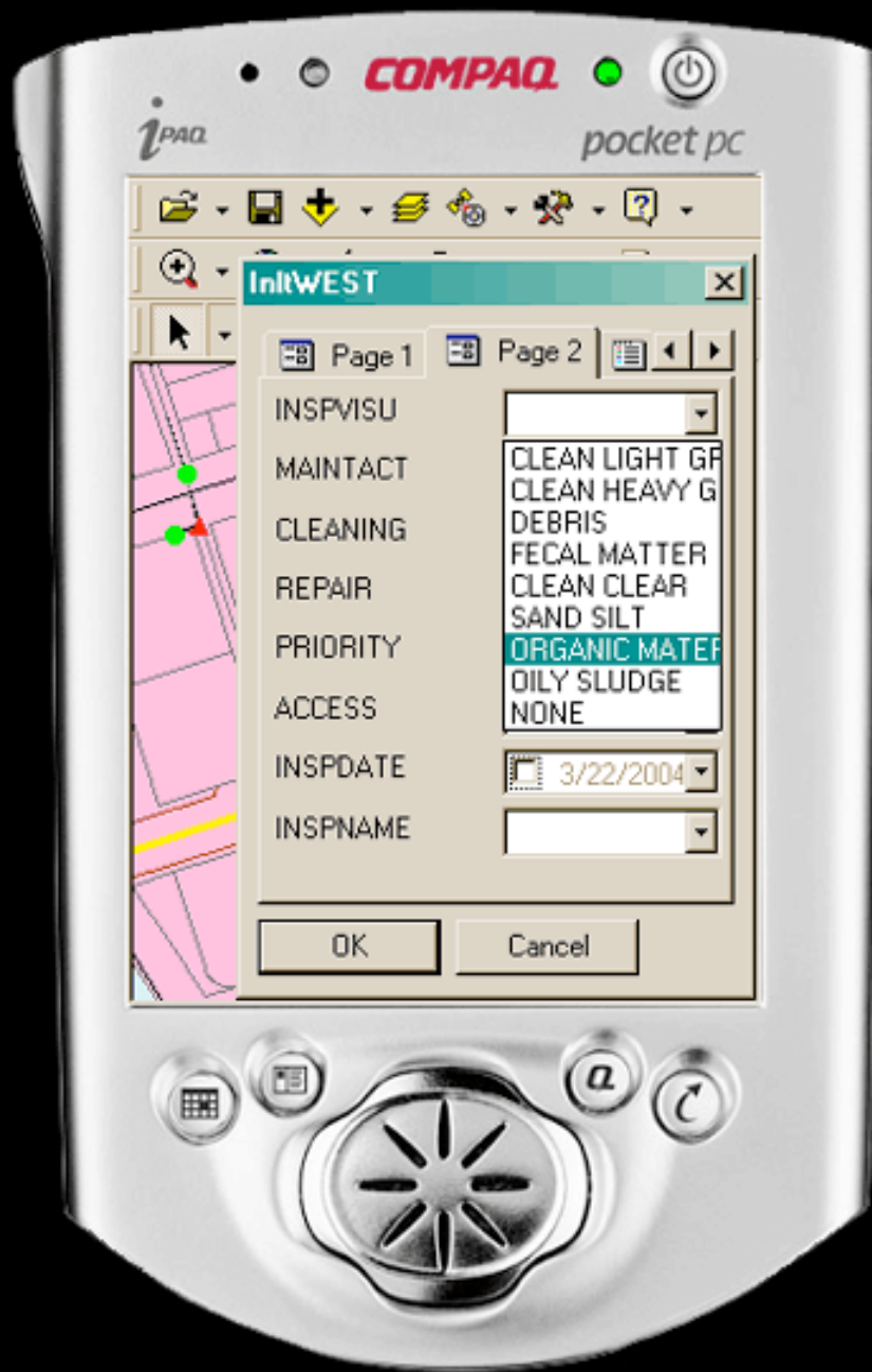
Page 2 of the form showing the visual inspection pick list
