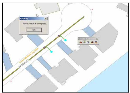
The **Sewer Lateral Tool** creates a sanitary sewer lateral between selected cleanouts and the closest sewer main. A dogleg is added in the downstream direction as well as the fitting whose diameter fields are transferred from the main.
