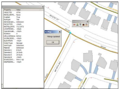
The **Fittings Tool** automatically populates up to four diameters from pipes to the Diameter1, 2, 3, 4 fields of intersecting pipe fittings, such as tees, bends, reducers, etc.
