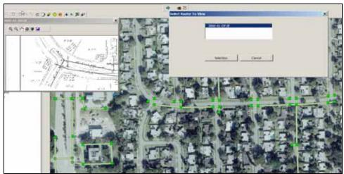
The **Storm Water Raster Tool** is an application that retrieves scanned images of source documents based on a user-defined polygon. It enables users to quickly reference engineering plan drawings within a defined geographic extent.
