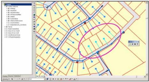
The **Water Service Lateral Tool** creates meters at the centroid of parcel polygons. This enables a rapid connection between utility infrastructure and the customer information system after geocoding the addresses attached to the parcels.
