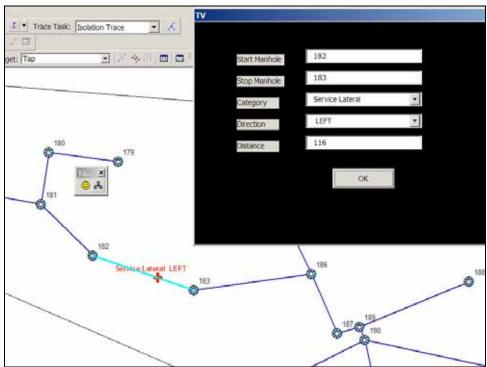
The TV Inspection Tool is an application that enables users to enter data from sewer TV Inspection logs including the start and stop manholes, the category (lateral, crack, root, etc.), right or left direction and the distance. The tool creates a point at the correct position.
