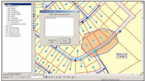
The **Roping Tool** automatically populates the SourceDocName and InstallDate fields for all utility infrastructure that is contained within the user-defined polygon. This speeds up the data conversion process.
