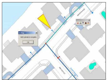
The **Water Service Lateral Tool** created service laterals connecting selected meters to the selected water main. This completes the connection between the water main and the customer information data that is linked to the meter.
