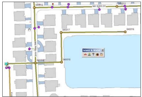
The **Sewer FacilityID Tool** populates the FacilityID field consisting of a reference to the downstream lift station and a 3-idgit sequence number – resulting numbers are labeled.
