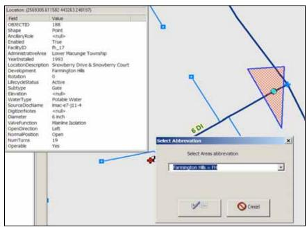
The **Valve Tool** populates a special FacilityID that is a concatenation of a development abbreviation and a valve sequence number. This creates a unique facilityID (in this case fh\_17) for valves when legacy valve numbers are repeated for each development.
