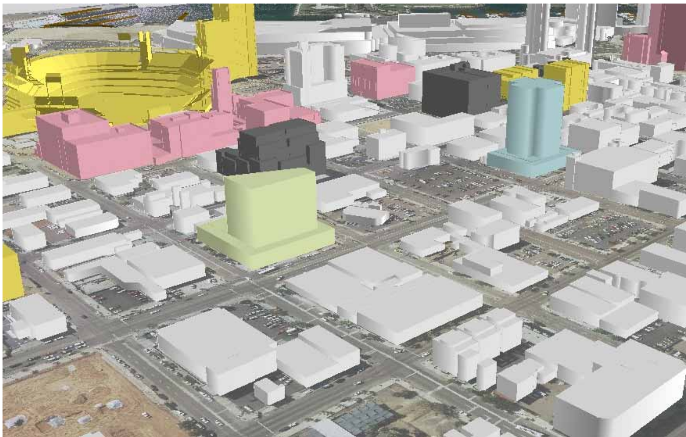
User created Scenarios rendered in 3D through ArcScene (red and yellow projects are proposed and under construction CAD models, green and blue are virtual projects)
