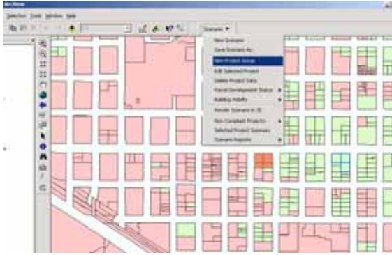
Scenario Builder Toolbar that activates VBA macros after virtual project parcels have been selected
