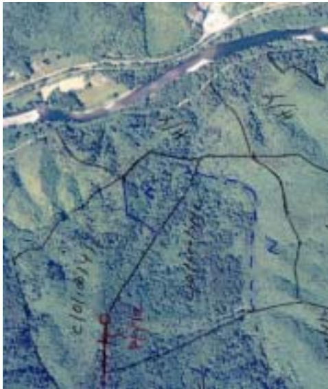
Figure 5. Portion of Conceptual logging and transportation plan, showing unit polygons and polygon attributes (black), proposed road locations and attributes (red), and non-thinnable polygons (blue).
