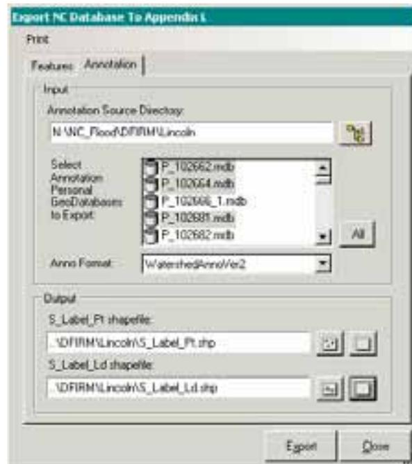
The output shapefiles for the FEMA Standard S\_Label\_Pt and S\_Label\_Ld can be created automatically from scratch, or the output from individual (or a set of) Personal Geodatabases may be appended to existing FEMA Standard annotation shapefiles. The output is projected to North Carolina State Plane, NAD83 Feet, FIPS 3200.
