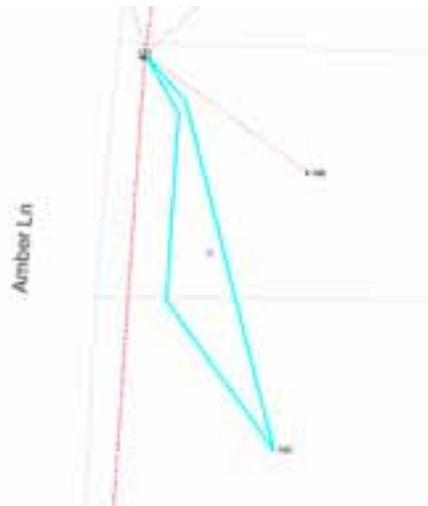
The most common error you will have when using this tool will be where the end points of the polyline match up. This is different than a loop as I will show you shortly.
