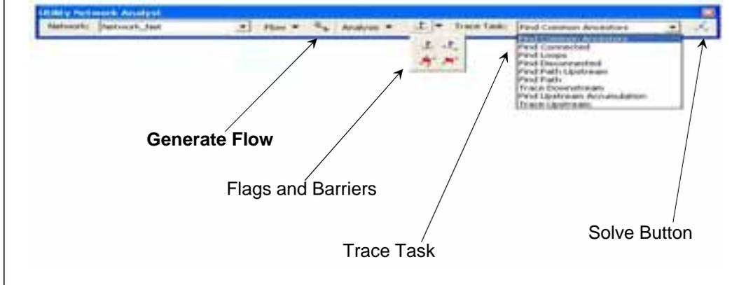
The final step to take before you can start to use your Geometric Network, or check for errors is to Set Flow Direction.
