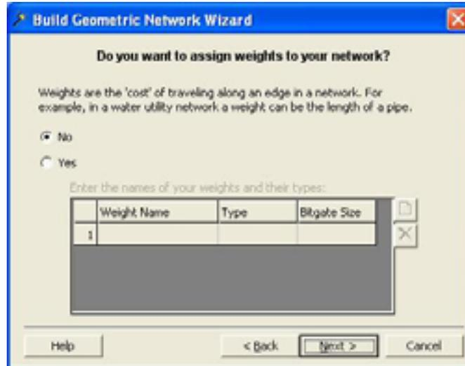
Weights are generally used for road, sewer, or water networks where resistance plays a factor.
