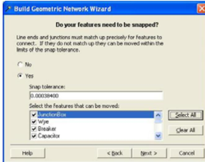
Snapping is a critical part of the wizard. All features need to be connected for this to work. Even if the ends of two lines are only a centimeter apart you cannot establish flow.
