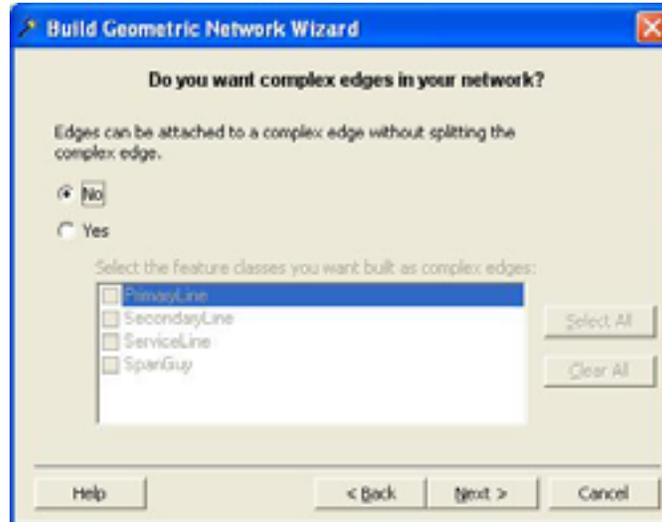
A complex edge allows features to connect without breaking a line. As long as one of the features has a node
