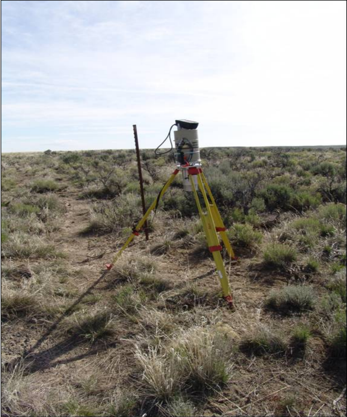
Figure 7: High Purity Germanium Detector used to measure Cs137 in soils
