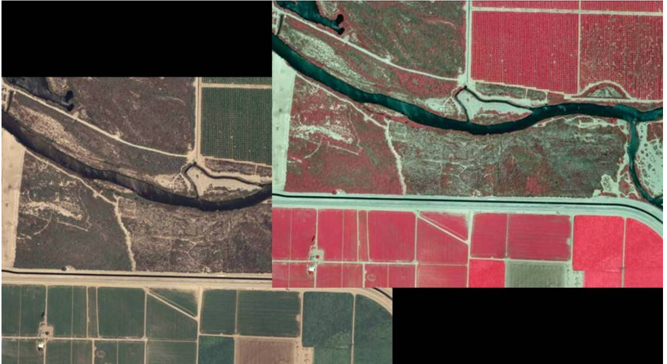
Figure 14: Natural color (left) and color infrared versions of the same area; from the Arizona 2007 four band project.
