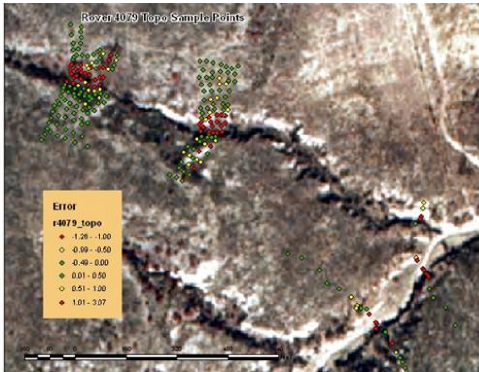
Figure 4. High accuracy GPS points collected using rover unit 4079 across an arroyo in Dawson Co. TX.
