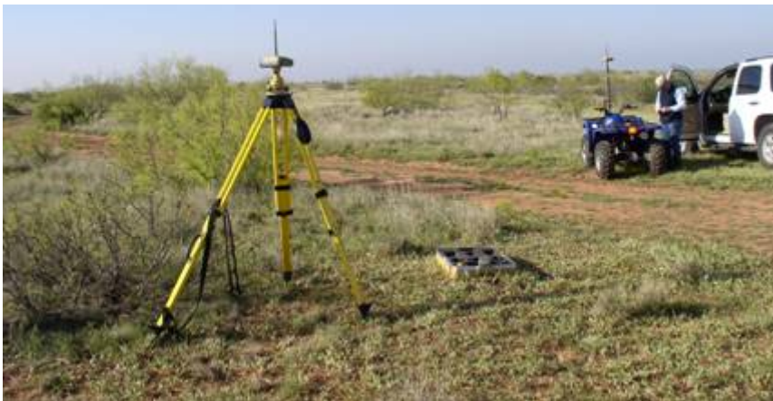
Figure 2. High accuracy GPS base station and ATV mounted Rover antenna setup at the Borden County evaluation site.
