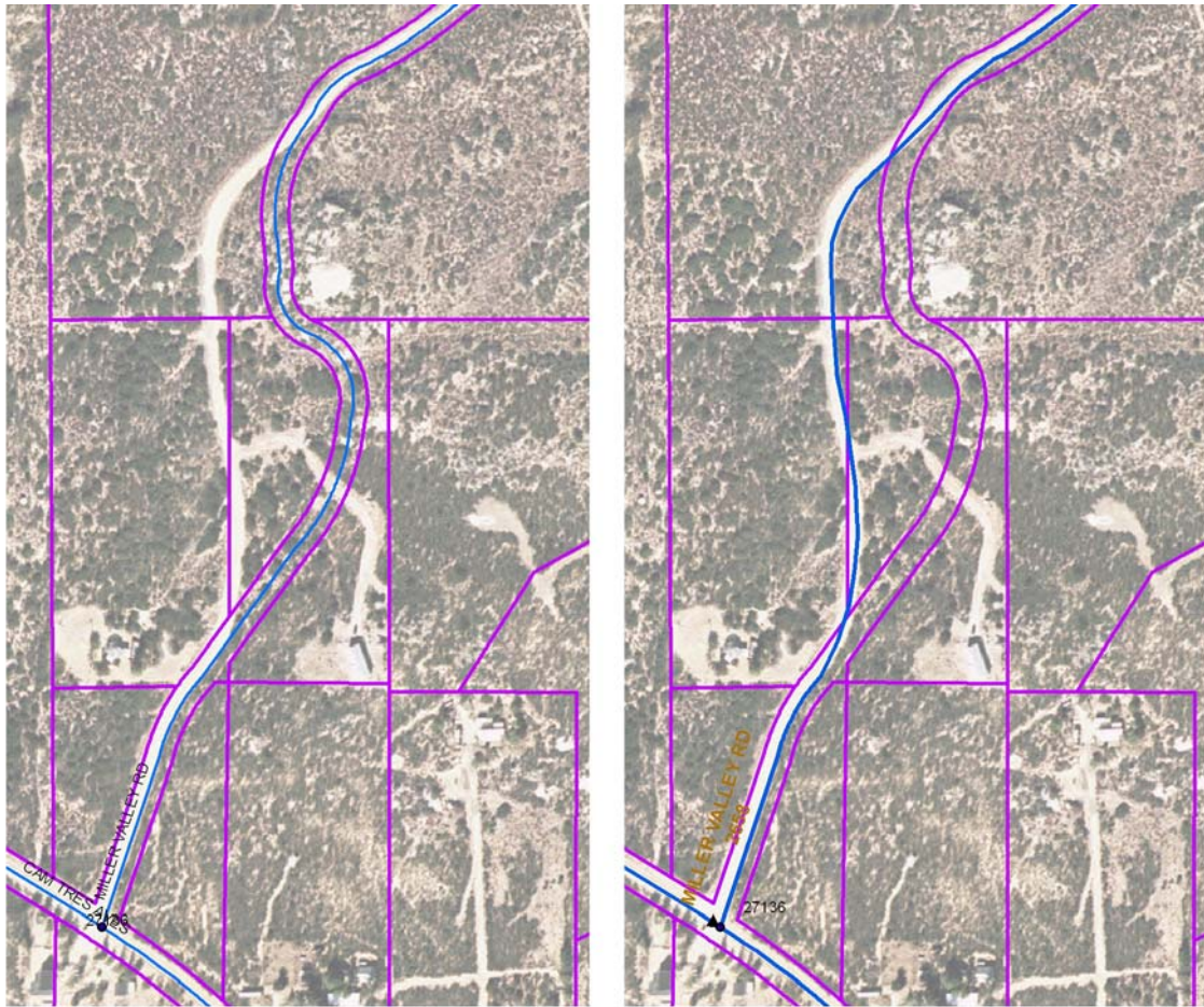
Figure 3: Left panel shows how road on aerial photo does not match vector data. Right panel shows road centerline edited to match reality.
