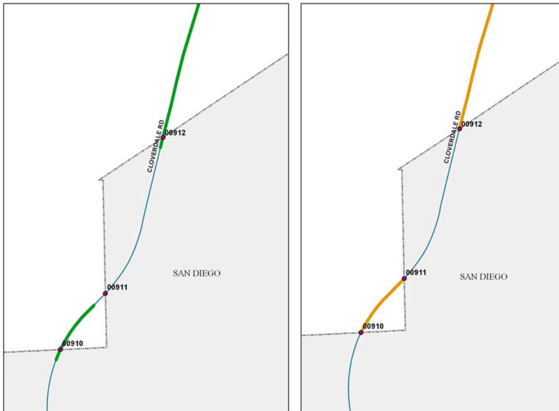
Figure 5: Example showing a route event for maintenance status. The County maintains the road in the unincorporated area, but not in the City. The uncalibrated route on left yields an incorrect map, with maintained portions shifted about 180 ft. Calibrating the route corrects the route event to properly match the City boundary.
