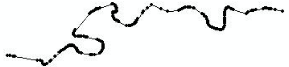
Figure 10 – Simplified line representation using BEND-SIMPLIFY algorithm and 20 m parameter among vertices – Number of resulting vertices: 147
