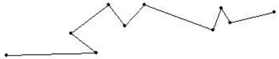
Figure 8 – Simplified line representation using POINT-REMOVE algorithm and 20 m parameter among vertices – Number of resulting vertices: 9
