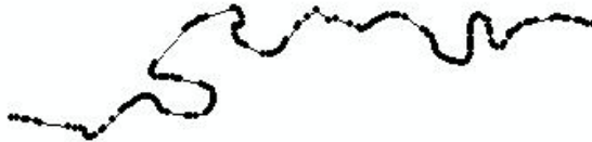
Figure 9 – Simplified line representation using BEND-SIMPLIFY algorithm and 10 m parameter among vertices – Number of resulting vertices: 171
