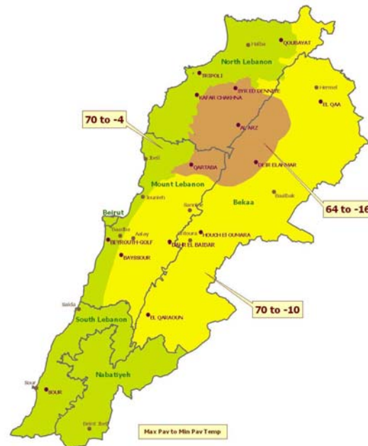
Figure 6: Proposed Pavement Design Temperatures for Lebanon
