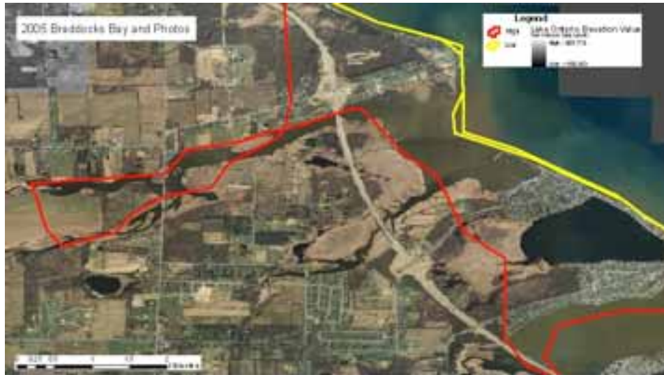
Figure 9- The 2005 analysis overlaid on the 2005 New York State Orthoimagery. As you can see large portions of the shoreline are supposed to be inundated and while there is problems with erosion, there is not a problem with complete flooding.
