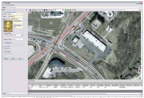
High-resolution ortho photos and CAGIS GIS data support detailed display of the location of interest. Here, CagisAIM is used to review an existing fire hydrant. The review form is integrated in the mapping interface to create a user-friendly platform in the field.
