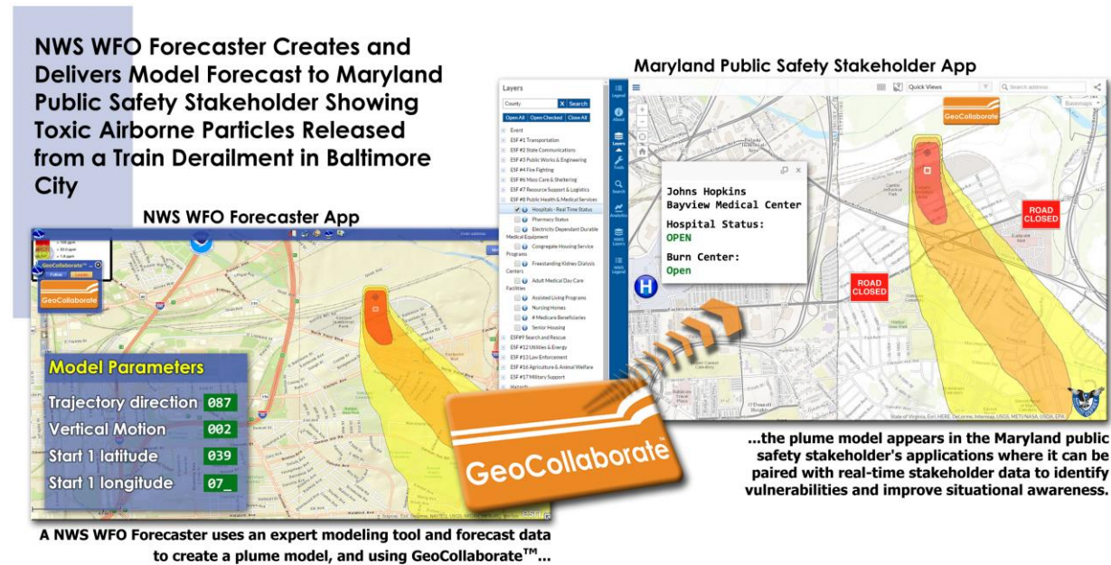
Fig 1- A HYSPLIT model run on an NWS office desktop PC showing airborne toxic materials from a train derailment shared within seconds with emergency managers on their web map applications using GeoCollaborate.
