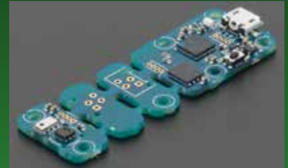
Reports ambient temperature, relative humidity & barometric pressure
