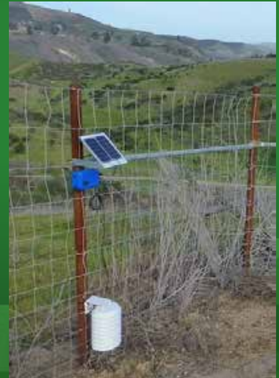
Valarm & Yocto-Meteo with Solar Power
