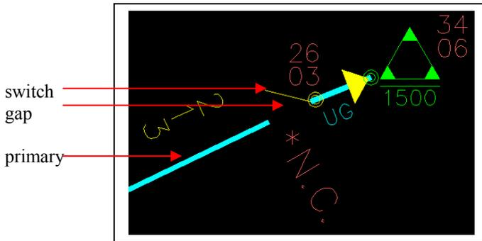
This DWG data indicates the physical gap in the primary with the inserted switch. During the conversion, this gap was closed to make a continuous primary line.
