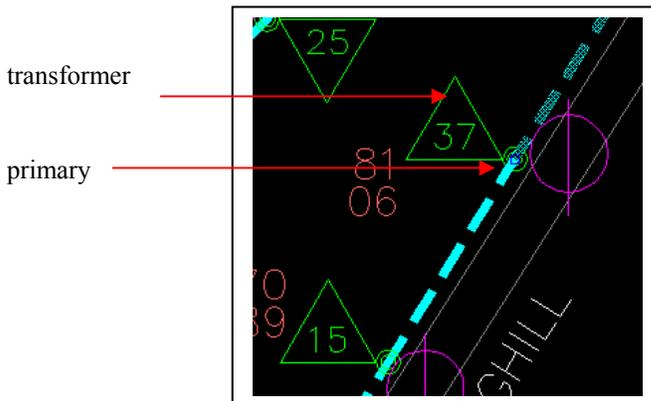
This DWG data shows the primary as the dashed line. The upper portion of the line is selected to show that there are two physical pieces of lines. But, having two separate lines is unnecessary because the attributes of the primary are the same on both sides. During the conversion, the primary line was joined together.
