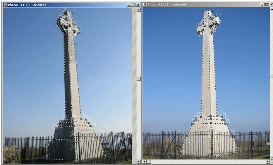
Figure 7: Mark and reference of common points for Tennyson's Monument, Isle of Wight.
