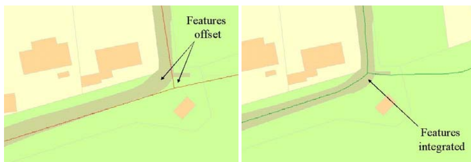
Figure 3. Integration of 1:25,000 path network to large-scale topographic data.
