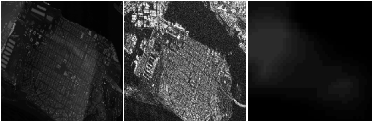
Figure 4: Comparison of digital elevation models. LIDAR data provided by Rapid Terrain Visualization, Fort Belvoir, VA. Radarsat R-Data © Copyright Canadian Space Agency 1999. All Rights Reserved © 2000 United States Government. DTED® is a registered trademark of the National Imagery and Mapping Agency.
