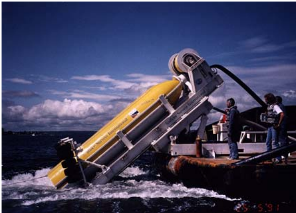
Figure 2a. The Sys09 instrument, owned and operated by Fugro Seafloor Surveys. Sys09 operates at 9/10 kHz is towed at ~100 meters below the sea surface. This instrument is used for surveying in 2,000 to 9,000+ meter water depth.
