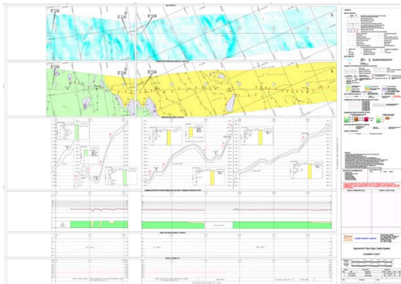
Figure 4b. An alignment sheet produced for a burial assessment. The top two panels show bathymetric contours and geologic interpretation in plan view. Note that the boxes are cut at each change in bearing of the route and rotated in an east-west direction so that the altitude views below (bathymetric profile, resistivity measurements, subsurface composition based on these measurements, and plough tow force estimates) will directly correlate to positions on the plan view boxes.
