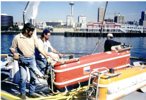
Figure 2b. The high resolution Sys100 instrument is employed for shallow water operations, in the 30 to 2,000 meter depth range. The instrument is towed near the seafloor, operating at a frequency of 100 kHz.
