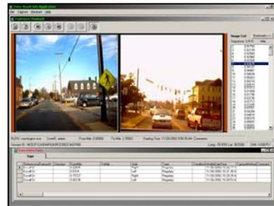
The Howard County Bureau of Highways (HCBH) performs pavement rating annually to determine its road maintenance budget. A video based asset-tracking solution was required to create and register digital images and voice descriptions to the county GIS road layer.
