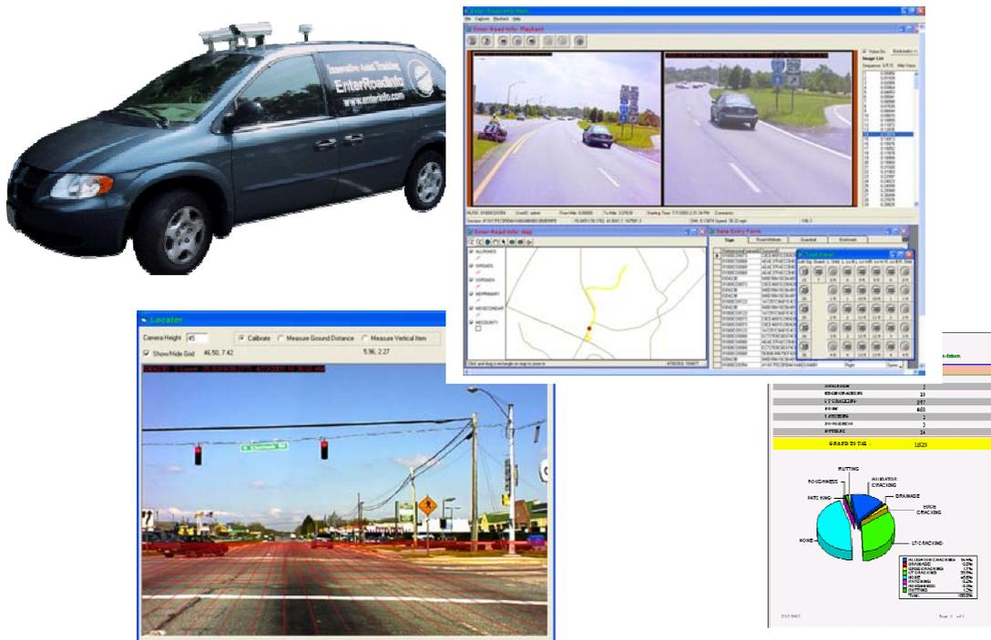
For the Charles County road inventory project, EnterRoadInfo was used to collect the road and sign attributes include county MUTCD type signs, number of lanes, and widths of the
