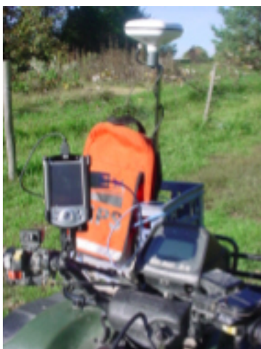
Figure 3. Handheld mobile data collection device mounted on ATV with GPS. (Photo source: Elizabeth Cook, GIS Specialist, NRCS, MO)
