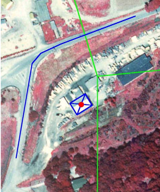
Figure 2: A control point (red) placed near the perimeter of an image's effective area (green). Sketching (blue) helps to precisely position control points.
