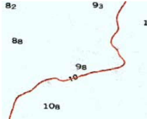
Figure 9. A bathymetry line extracted using Feature Analyst. The initial polygon results were converted to a line, jumping gaps where necessary, and the line was adjusted to the underlying raster.
