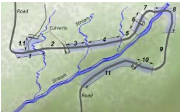
Figure 1. Determination of road segments happens in the field based on drainage and delivery of water. (WARSEM Manual, WADNR, 2004)
