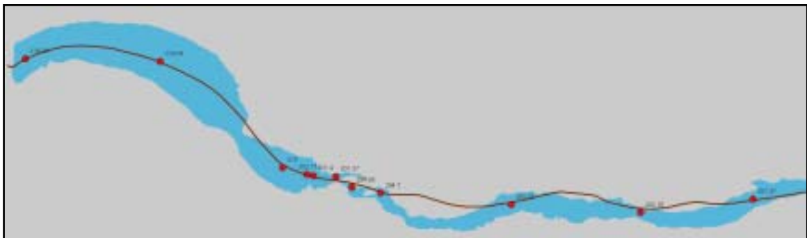
Fig 3. shows the digitized water polygon, the flight path, and control points with elevation labels
