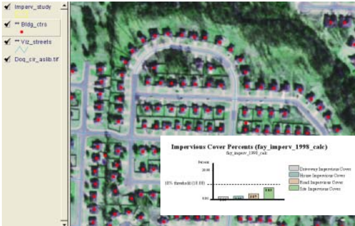
Figure 1: An example of the Impervious Surface Scenario that includes the actual Indicator Chart of impervious surface summary.
