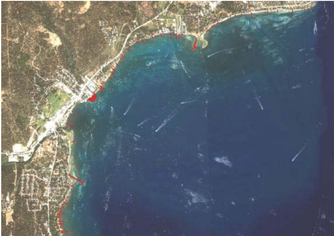
Fig. 8: Results of mapping piers (shown in red) from IKONOS data for the Dollar point area.
