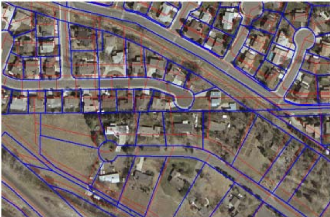
Figure 2. Unrectified parcels in red, Rectified parcels in blue on 2002 aerial imagery disparate data themes for the entire County into synchronization to enable a final
