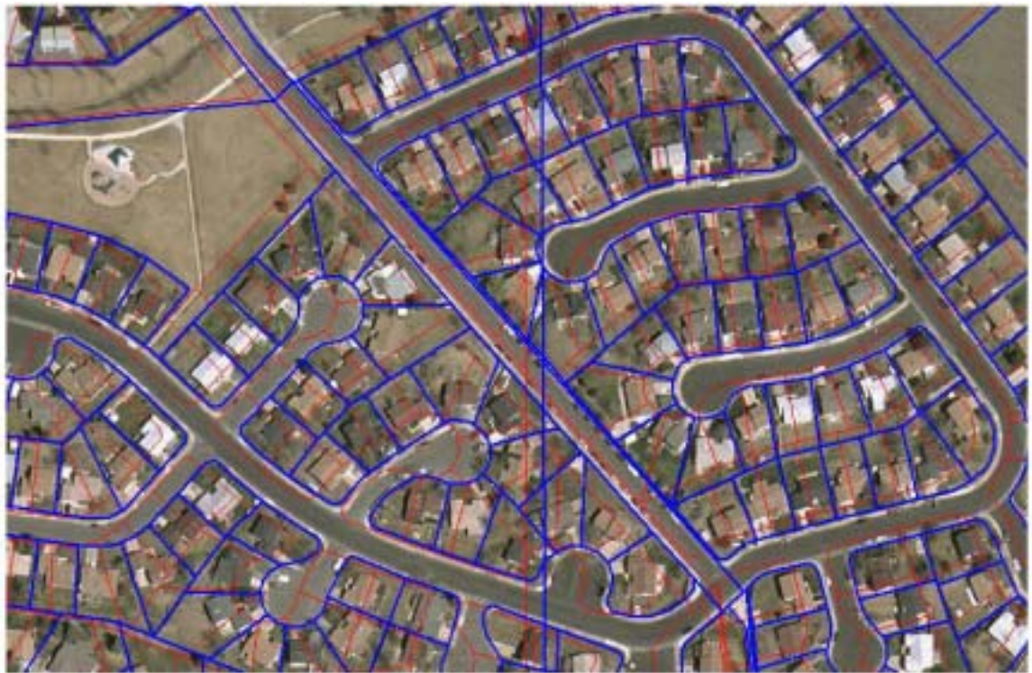
Figure 4. Parcel after rectification in blue, parcels before rectification in red on 2002 aerial imagery. Note: The shift correction is in many directions relative to the image.
