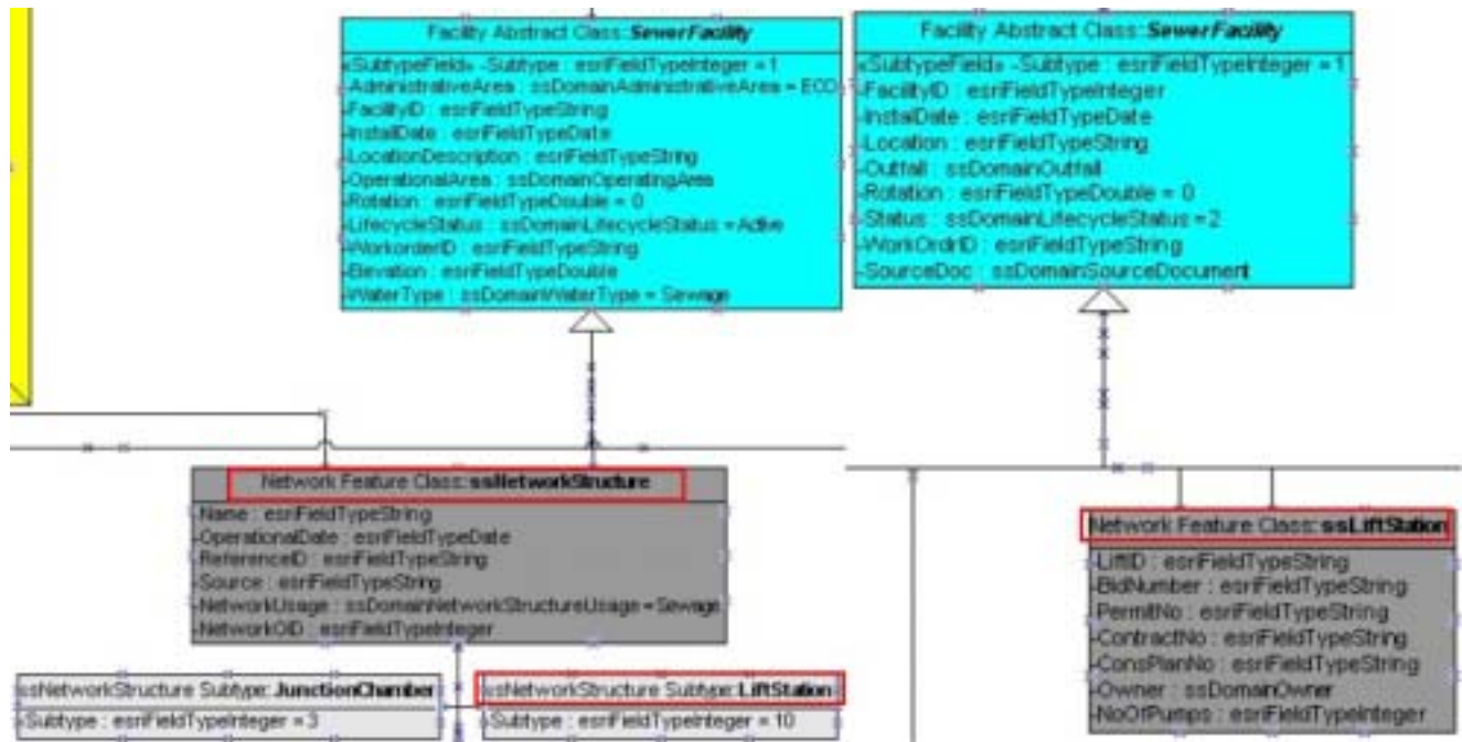
ESRI Model Customized Torrance Model Diagram Showing Differences between ESR Sewer Facility Model and Torrance Sewer Facility Model
