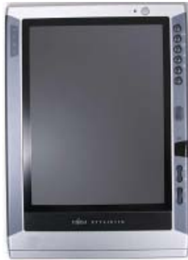
Figure 1. A mobile field computer. This computer has external USB ports for connecting data capture peripherals such as digital cameras and GPS.
