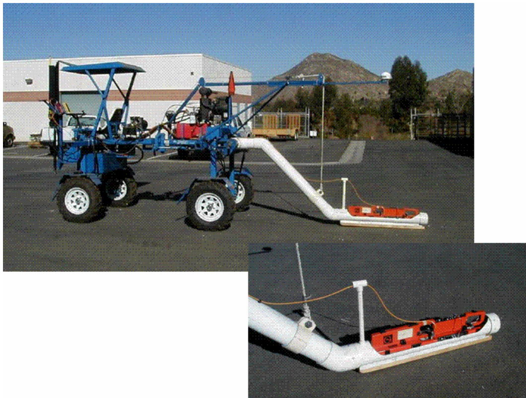
Figure 4. Mobile GPS-based electromagnetic induction (EMI) equipment showing (a) a side view of the entire rig and (b) a close-up of the sled holding the EMI unit.
