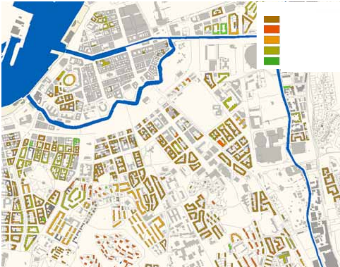
Figure 5. Energy model based on energy statistics for blocks of flats. The average energy use is illustrated based on SCB-data (1999) in kWh/m 2 *year in age-classes, i.e. year of construction.
