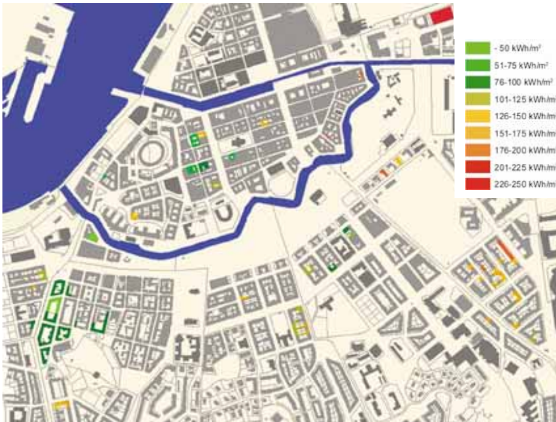
Figure 4. Energy model illustrating the energy use in kWh/m 2 *year for heating and hot water for buildings owned by three real-estate managers in Goteborg. The reference year is 2000. The grey marked properties are not owned by them.
