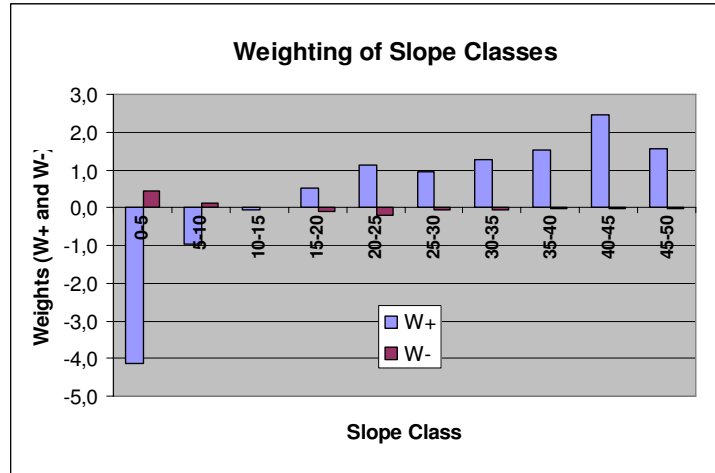
Fig. 7: Slopes between 20 and 50 % are significant indicators for landslides, while slopes lower than 15 % are a secure indication for the absence of landslides.
