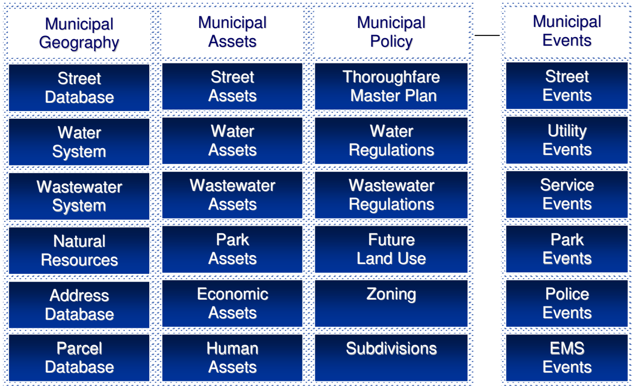
Figure 2. Diagram of Typical Data Components of a Comprehensive Centralized GIS
