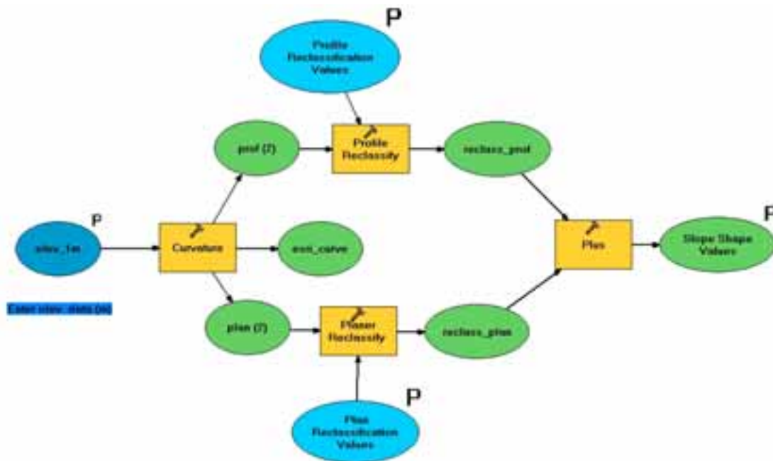
Figure 3. Slope shape model. This model will produce a reclassified combination of the profile and planer curvature derivatives of an elevation dataset.
