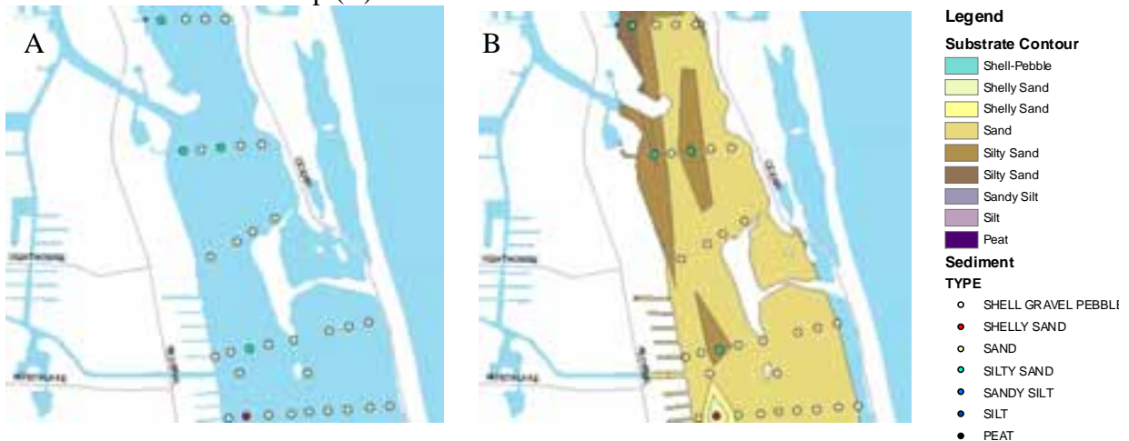
Figure 6. Digitized Substrate Characteristics from Sediment Cores and Muck Survey (A) and Substrate Contour Map (B)
